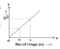
**GRAPH:** Plot a graph with square of diameter  $D_m^2$  on Y-axis and order of the ring m on X-axis. Slope of this graph is  $4\lambda R$ . Hence wavelength is  $\lambda = \frac{slope}{4R}$
