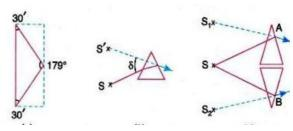
emanate from virtual source  $S_1$ . The bottom part deviates upward and appears to come from virtual
