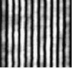
5. The fringe width is calculated using the formula  $\beta = \frac{x_n - x_0}{n}$
